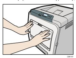
2. Pull Front Cover Open Lever, and then open the front cover with both hands carefully.
